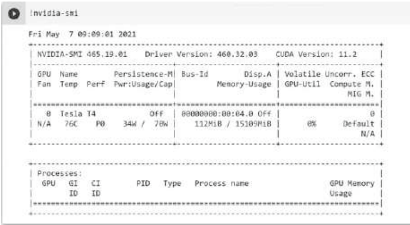
Fig. 11.4 The output of nvidia-smi command
