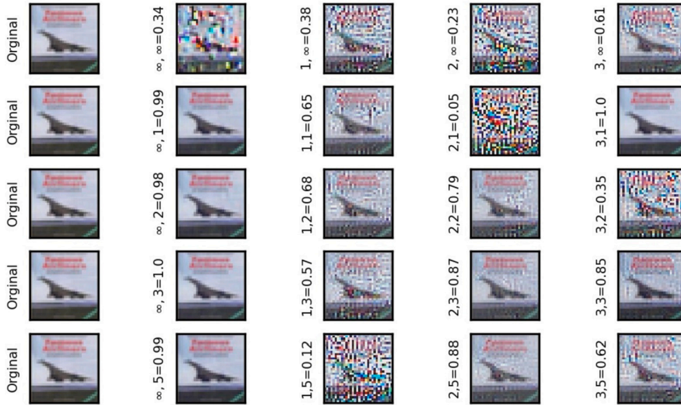
Fig. 5. DeepFool attack results on CIFAR10 for an airplane image sample. Title of each image indicates the value of T used for training ( T_{tr} ) and testing ( T_{te} ), followed by its SSIM score in the form of T_{tr}, T_{te} = \text{SSIM} . The images show the attack cannot make adversarial samples with low perturbation levels when binomial neurons are employed (apparently this is when T_{tr} > 1 ).
