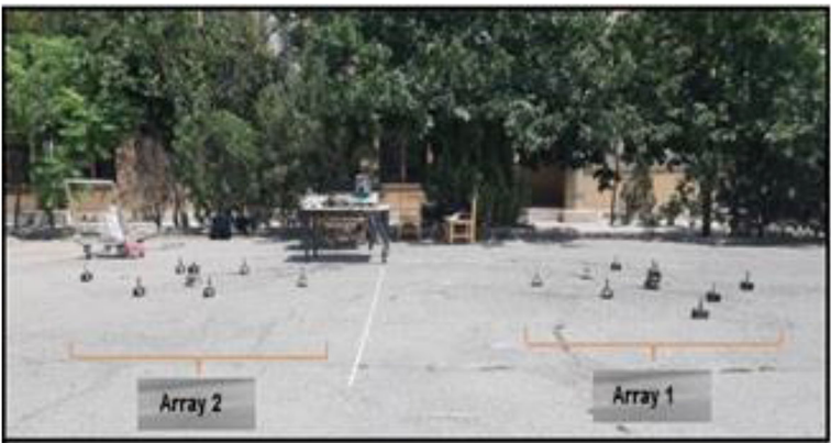
Fig. 4 The microphone array topology of Array 1 and Array 2 for outdoor testing
