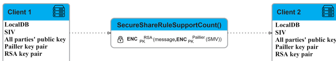
Fig. 5 Proposed communication protocol in our scheme
